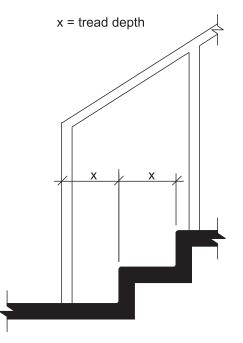
Fig. 505.10.3 Bottom Handrail Extensions at Stairs
