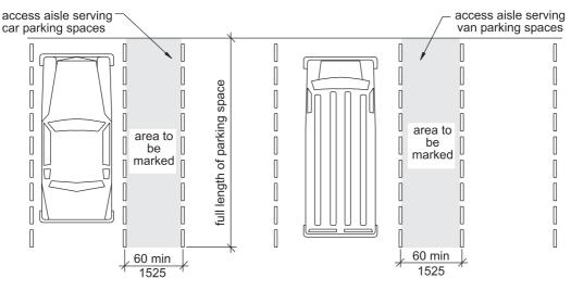
Fig. 502.4 Parking Space Access Aisle
