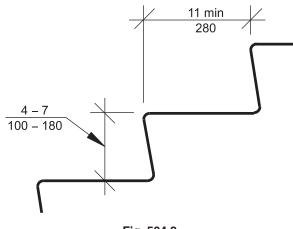
Fig. 504.2 Treads and Risers for Accessible Stairways
