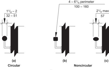
Fig. 505.7 Handrail Cross Section
