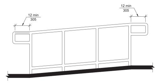
Fig. 505.10.1 Top and Bottom Handrail Extensions at Ramps
