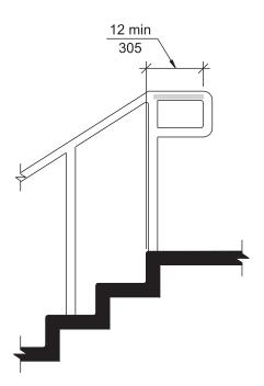
Fig. 505.10.2 Top Handrail Extensions at Stairs
